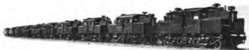
Ten of the thirty-five 100 ton 2200 horse-power electric locomotives built for the New York Terminal electrification of the New York Central Lines by the General Electric Company and the American Locomotive Company
